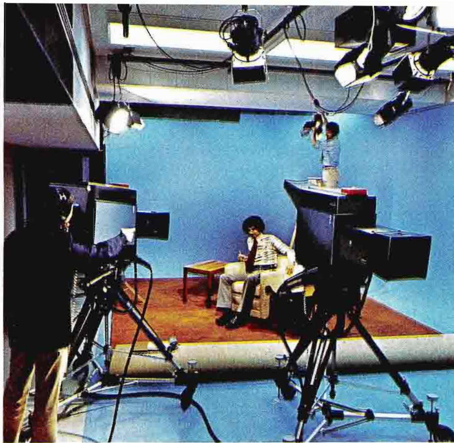
Setting up lighting for a studio production. Two TK-45A cameras are installed, one with a portable CCU for handling remotes.
