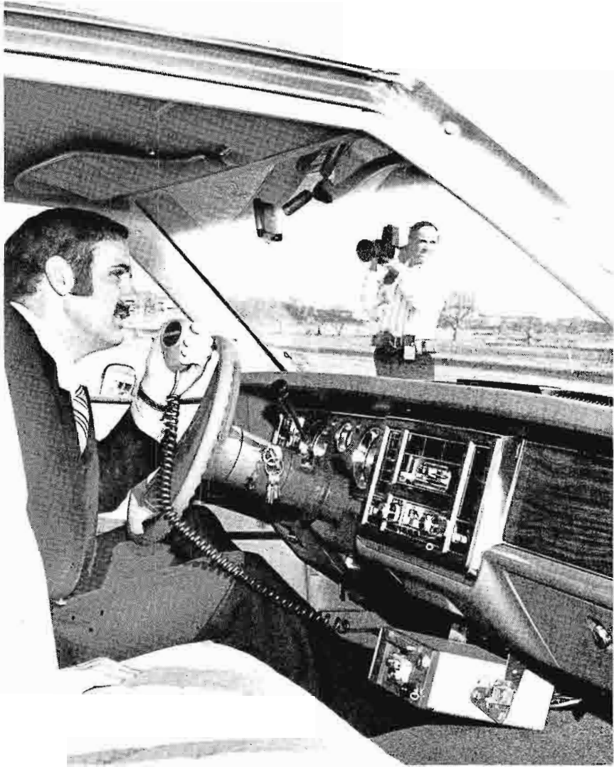
For greater coverage and communications versatility, TACTEC portable can also be used as a mobile radio with the addition of a vehicular charger and power booster.
